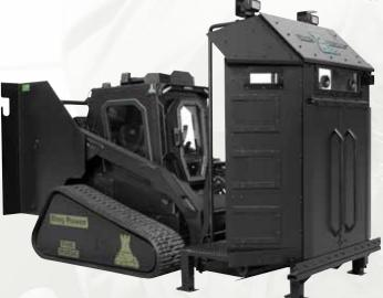
When the Armored Deployment Platform is mounted on the vehicle, the operator can raise it to 11 feet so that entry can be made on both the first and second floors, and the roofs. The platform height is also ideal for airplane assault incidents. In a vehicle take down, the platform can be slanted downward for crowd control and rescues.
